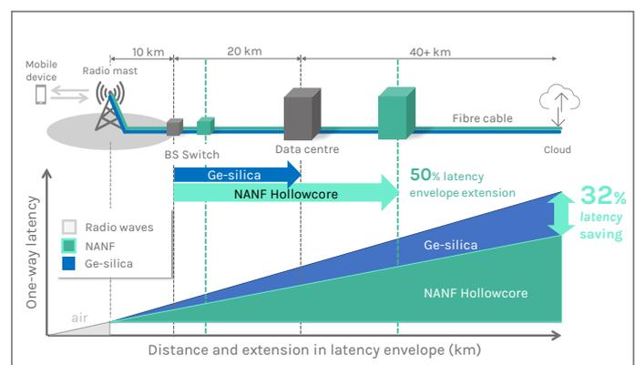
Figure 4: Signal path latency in cellular radio-fibre networks
