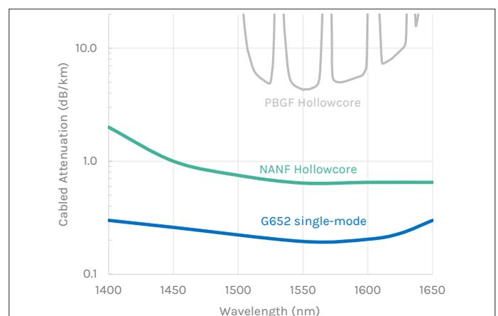
Figure 5: Comparison of spectral attenuation
