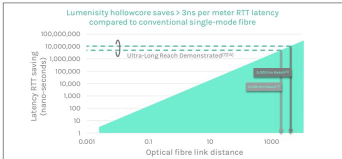
Figure 2: Latency of hollowcore compared to glass-core fibre
