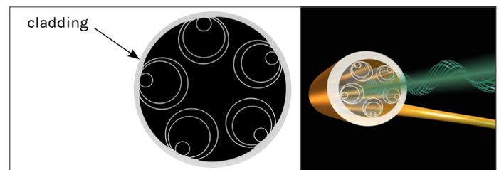
Figure 1: Cross-section the NANF structure and software model to illustrate light propagation and signal loss
