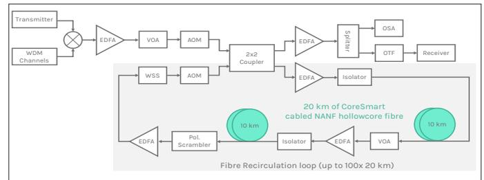
Figure 9: A recirculating loop was used to demonstrate 400Gb/s over more than 2,000 km of cabled NANF hollowcore fibre
