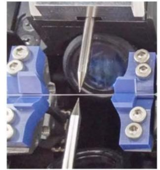
Figure 11: Field fusion splice capable using commercially available equipment
