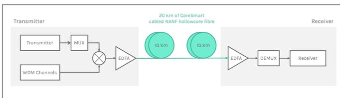
Figure 7: 20.5km point-to-point link demonstrating 19.2Tb/s & 38.4 Tb/s<sup>[2]</sup>
