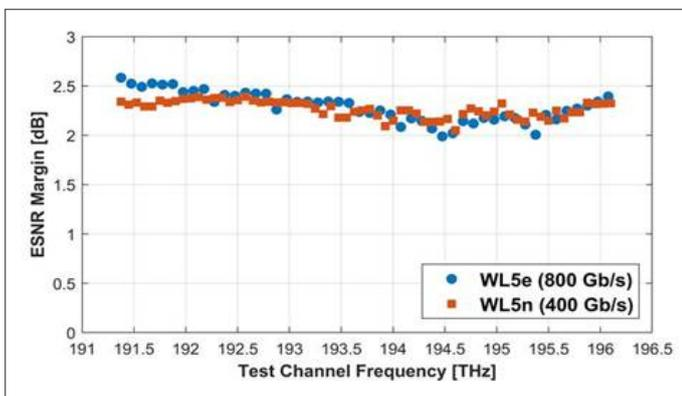
Figure 8: Plotted results showing ESNR vs Channel Frequency
