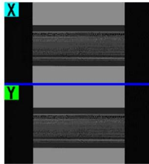
Figure 12: A splice machine screen image of fused NANF hollowcore fibre
