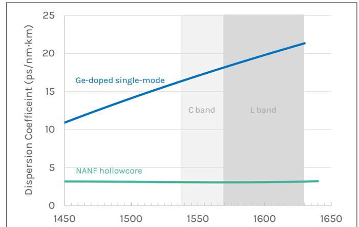
Figure 6: Comparison of chromatic dispersion (cabled fibre)
