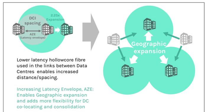
Figure 3: Lower latency DCI offers cost saving options enabled by DC Geographic expansion
