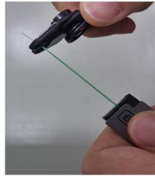
Figure 10: Mechanically strippable fibre coating
